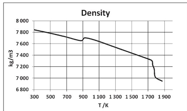
Figure 2 Density of AISI 1016 steel versus temperature [16]
