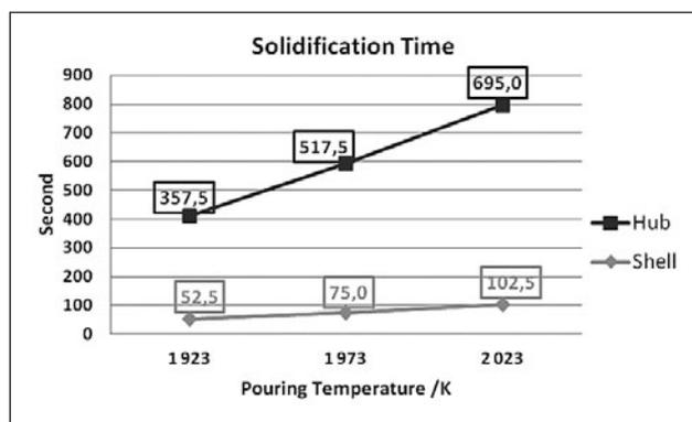
**Figure 14** Solidification time calculated at the author shell and the hub
