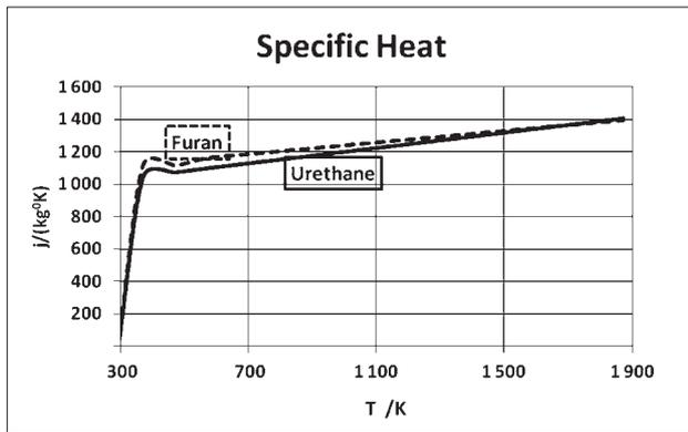
**Figure 4** Specific heat of urethane and furan bonded sand versus temperature [23]
