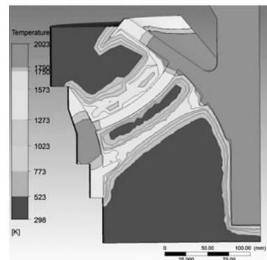
**Figure 13** Temperature contours in 60° segment of the impeller and the core at  $t = 90$  s ( $T_{\text{pouring}} = 2\,023$  K)
