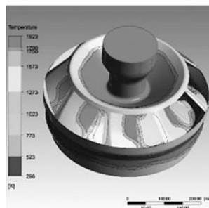
**Figure 9** 3D impeller at  $t = 45$  s ( $T_{\text{pouring}} = 1\,923$  K)
