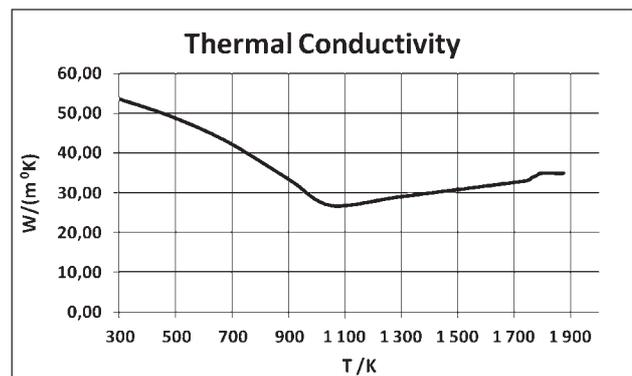
Figure 3 Thermal conductivity of AISI 1016 steel versus temperature [16]
