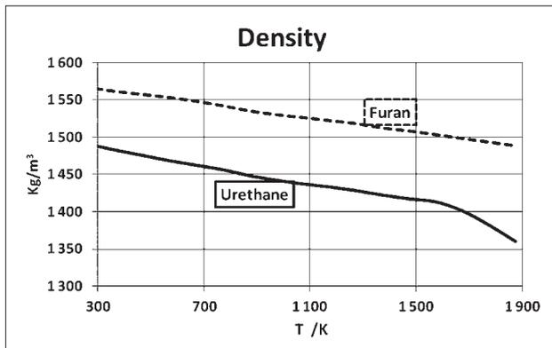
**Figure 5** Density of urethane and furan bonded sand versus temperature [23]
