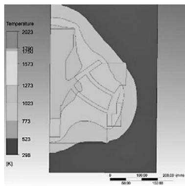
**Figure 15** Temperature contours in 60° segment of the impeller, the core and the mold at  $t = 7\,200$  s ( $T_{\text{pouring}} = 2\,023$  K)
