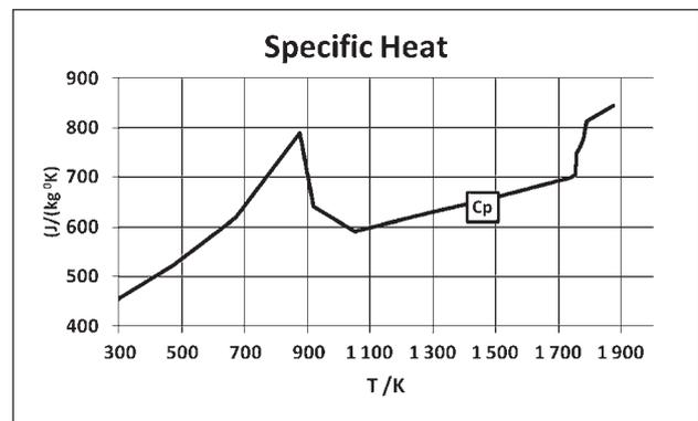
Figure 1 Specific heat graph of AISI 1016 steel versus Temperature [16]
