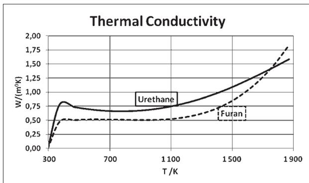
**Figure 6** Thermal conductivity of urethane and furan bonded sand versus temperature [23]
