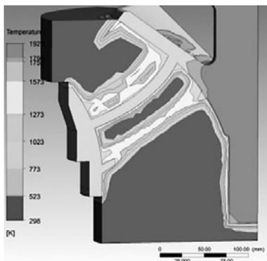
**Figure 12** Temperature contours in 60° segment of the impeller and the core at  $t = 60$  s ( $T_{\text{pouring}} = 1\,923$  K)
