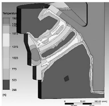
**Figure 11** Temperature contours in 60° segment of the impeller and the core at  $t = 45$  s ( $T_{\text{pouring}} = 1\,923$  K)
