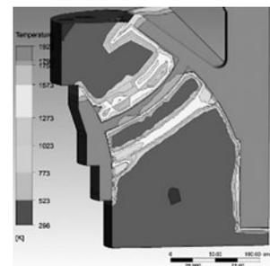
**Figure 10** Temperature contours in 60° segment of the impeller and the core at  $t = 25$  s ( $T_{\text{pouring}} = 1\,923$  K)
