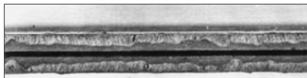
Figure 4 The influence of uneven distribution of oxygen in the material on the penetration by the length of weld
