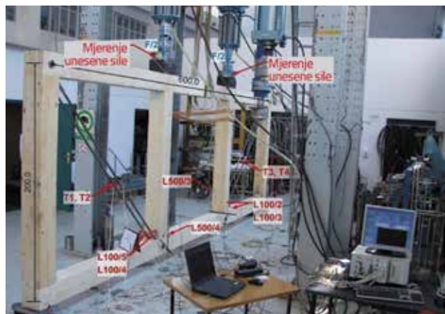
Figure 2. Experimental testing of trusses
