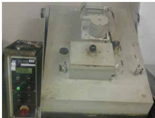
Figure 2. Laboratory asphalt mixer
