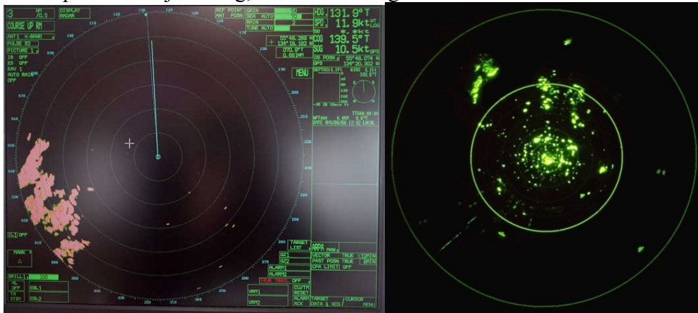
Figure 9 Camouflaging the location of the ship in noise jamming Slika 9 Maskiranje pozicije broda u šumu smetnje
