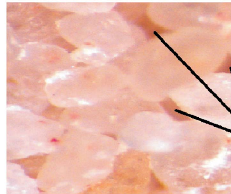
Fig 3. Almost unconsolidated to semi-consolidated sandstone sample illustrating the lack of cement with perfect homogeneous grain size with a uniform distribution and the high roundness level, Magnification: 64, Focus: 8.95 mm, Field: 3.6 mm, Porosity = 30%, Permeability = 1 761.27 mD.
