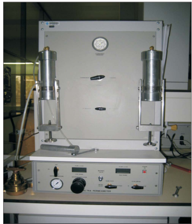
Fig 6. Ultra Perm 400™ used for measurements of permeability ( k ) at KACST Research Center Sl. 6. Ultra Perm 400™ korišten za mjerenja propusnosti ( k ) u istraživačkom centru KACST
