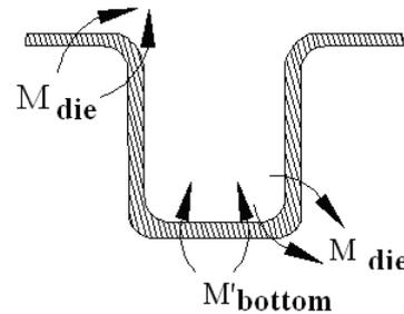
b) Springback caused by hot contact bending
