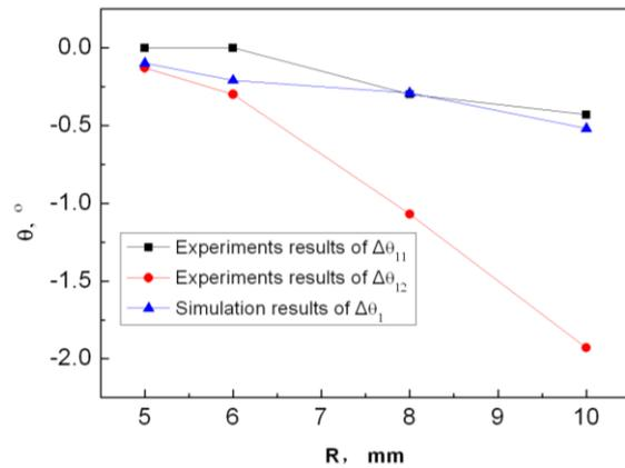
Figure 6. The relationship between the die radius and springback  $\Delta\theta_i$ .
