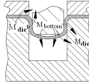
a) Springback caused by the forming force
