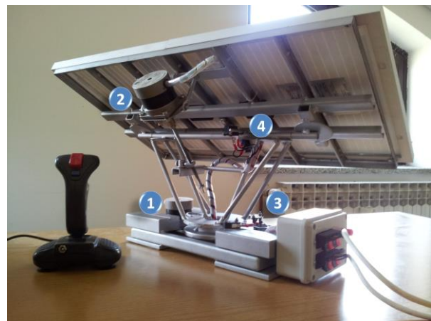
Figure 7. Real dual-axis tracking system
