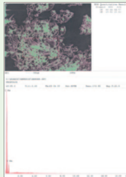
Figure 6 Elemental chemical analysis of the sample of the nature propolis preparation for the presence of heavy metals, performed on electron microscope SEM Philips XL 30 with EDX detector (EDAX), with 10mm 2 of active surface (Centre for forensic investigations, research and expertise Ivan Vučetić, Zagreb, Croatia)
