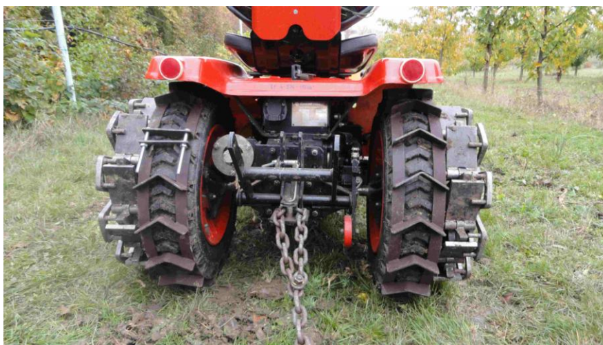
Figure 4: Wheels equipped with auto-extensible blades and steel boots mounted to the tractor rear wheels
