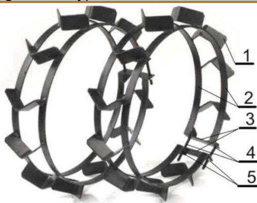
Figure 3: Steel boots: 1 – traction strip, 2, 3 – strips, 4, 5 – clamping with two clamping screws with M10 nuts
