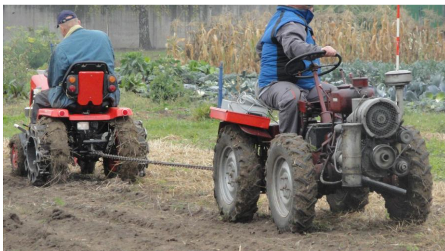
Figure 6: Measurement of drawbar pull
