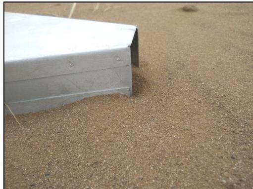
Figure 4. Reduction of transverse profile of device due to soil accumulation
