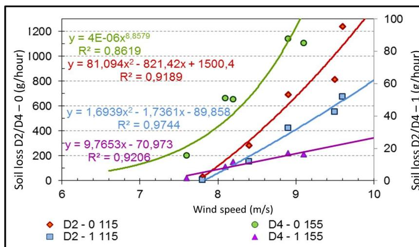
Figure 3. Graph of measured soil erosion in the D2 and D4 from the day 30.3.2012 and their regression equation
