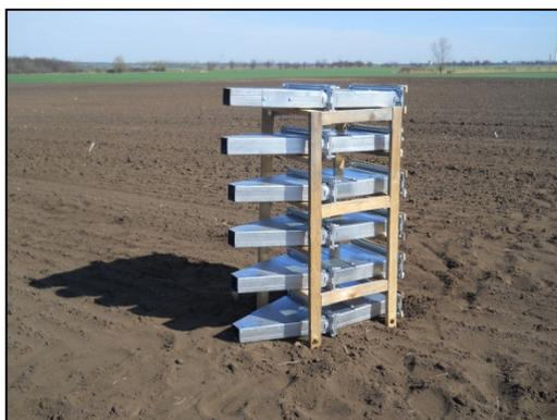
Figure 1. The prototype of soil particles catcher
