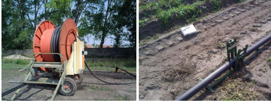
Fig. 2: Bauer Rainstar 90/300 TX Plus irrigation machine with Ecostar 4000, field measurement
