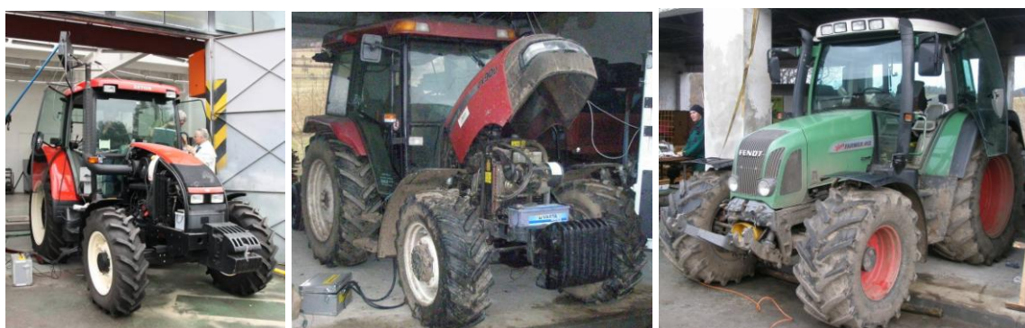
Figure 2: Measured tractors: a) Zetor Forterra 8641 – max. power 61 kW, max. torque 353 Nm, b) Case IH JX 90 – max. power 80 kW, max. torque 382 Nm, c) Fendt Farmer 412 Vario – max. power 93 kW, max. torque 622 Nm
