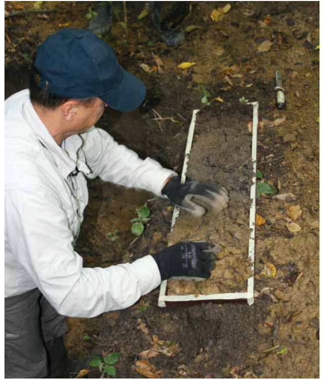
Slika 8. Prenešeni monolit tla Figure 8 Soil monolith carries over
