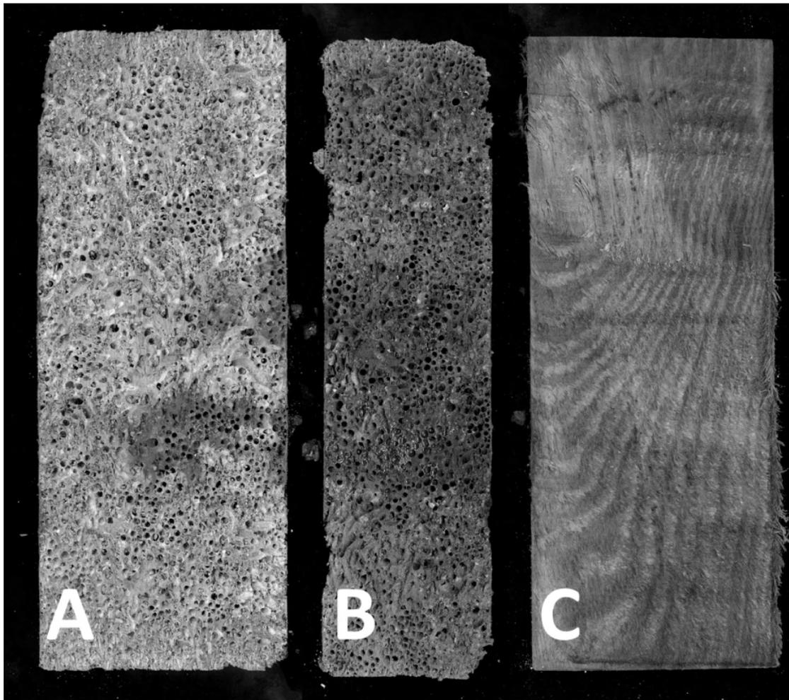
**Figure 2** Cross-sections of specimens exposed in the Port of Koper: (A) untreated Scots pine sapwood and (B) untreated sweet chestnut heartwood exposed for 10 months; (C) Scots pine sapwood impregnated with Silvanolin C ( $c_{Cu} = 1.25\%$ ) exposed for 32 months
