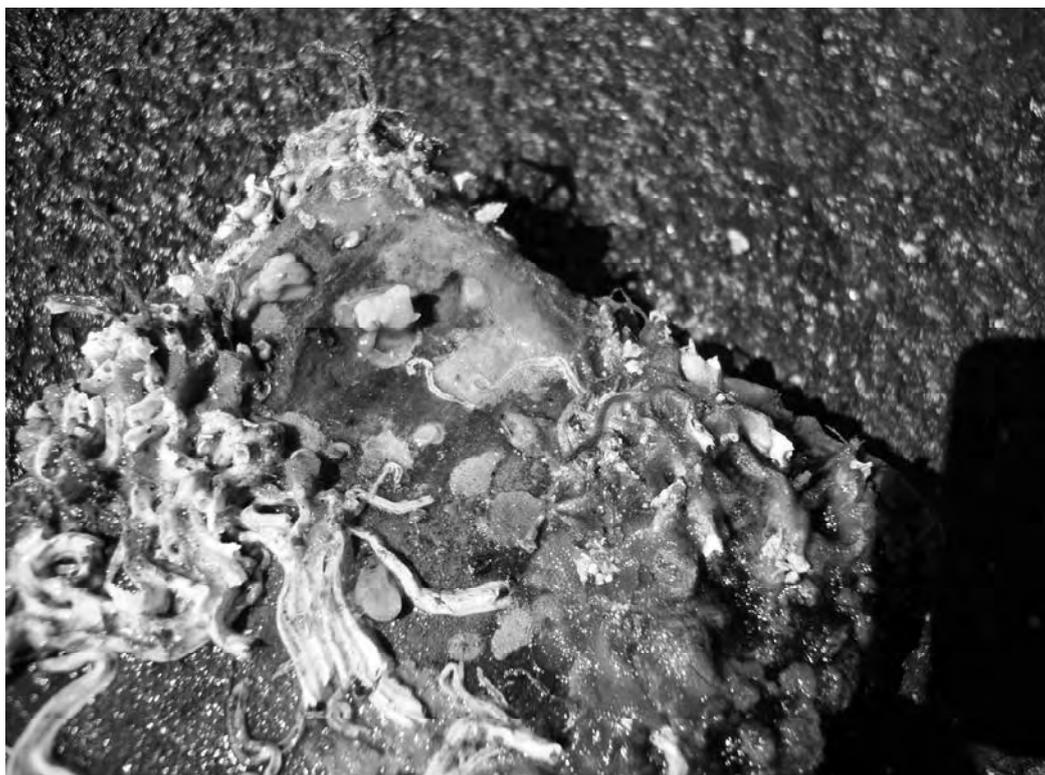
**Figure 1** Visual appearance of specimens after 10 weeks of exposure in Adriatic Sea
