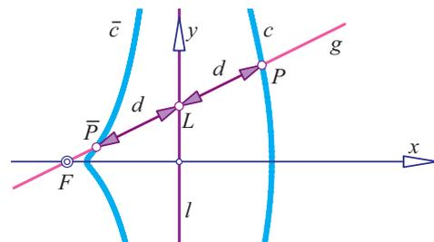
Figure 1: The construction of the conchoid  $c$  of a line  $l$  in the plane.
