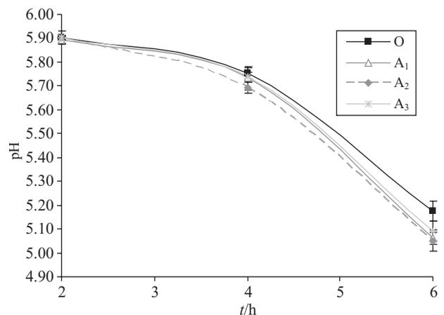
**Fig. 3.** Acidification activity of *L. plantarum* 564 cells before and after the PEF treatment, incubated in MRS broth at 37 °C during 24 h after the treatment. O=control (untreated) sample; A<sub>1</sub>, A<sub>2</sub> and A<sub>3</sub>=PEF-treated samples with the applied energy of 1.33, 5.5 and 12.2 J/cm<sup>3</sup>, respectively
