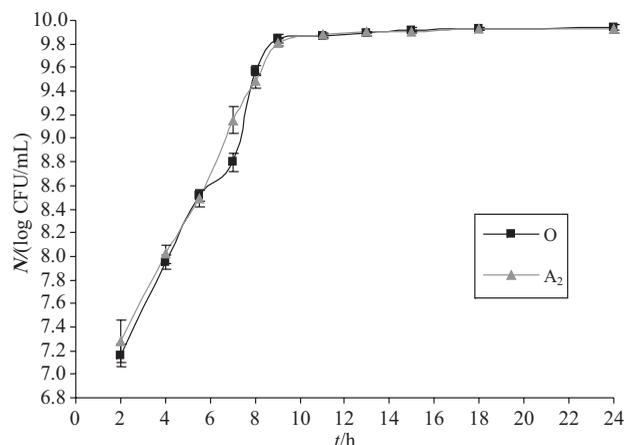
Fig. 1. The growth of *L. plantarum* 564 cells before and after the PEF treatment, incubated in MRS broth at 37 °C during 24 h. O=control (untreated) sample, A<sub>2</sub>=PEF-treated sample with the applied energy of 5.5 J/cm<sup>3</sup>
