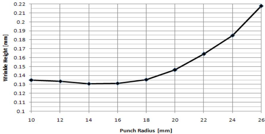
Fig. 10 The effect of varying punch radius on wrinkle height
