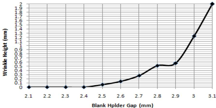
Fig. 9 The effect of varying blank holder gap on wrinkle height
