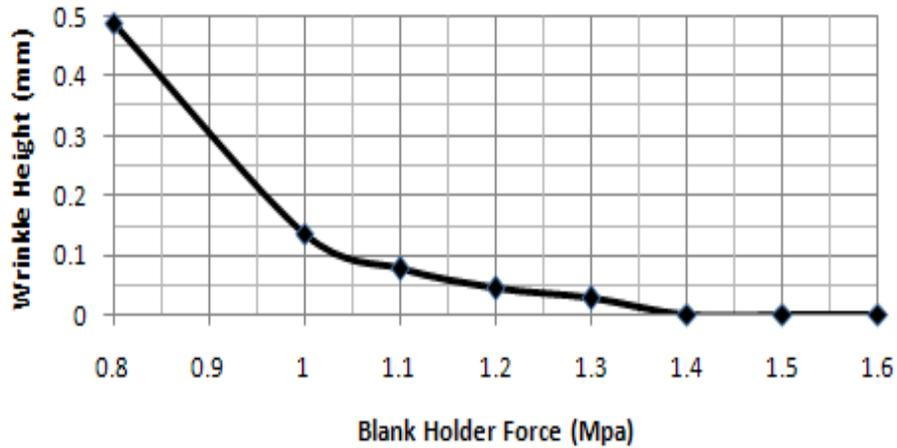
Fig. 6 The effect of different blank holder forces on wrinkling for AA5754-O aluminium alloy
