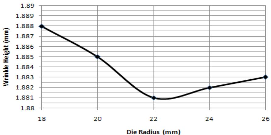
Fig. 12 The effect of varying die radii on wrinkle height for radii above 18mm
