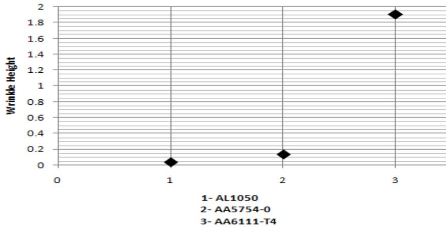
Fig. 4 The effect of wrinkling on different types of aluminium alloys
