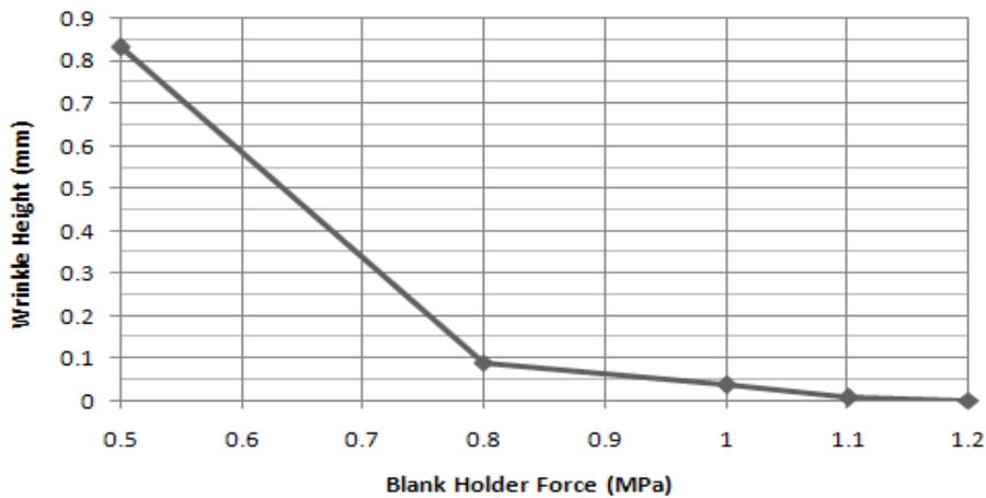
Fig. 7 The effect of different blank holder forces on wrinkling for Al-1050 aluminium alloy
