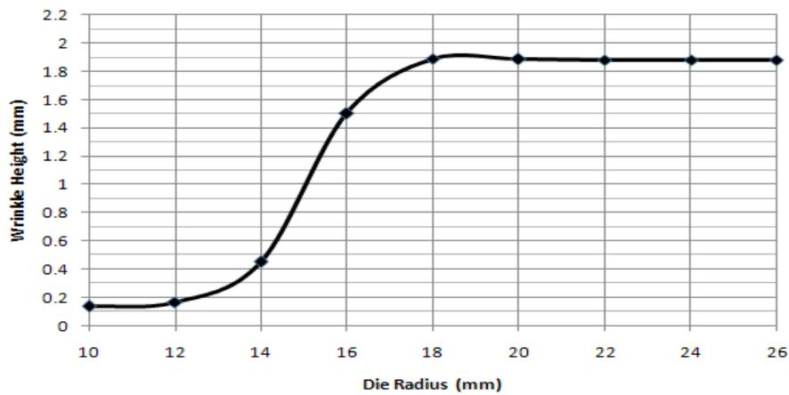
Fig. 11 The effect of varying die radii on wrinkle height
