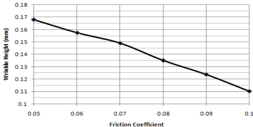
Fig. 13 The effect of varying friction coefficient on wrinkle height
