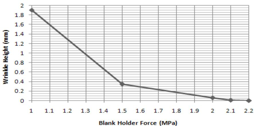
Fig. 8 The effect of different blank holder forces on wrinkling for AA6111-T4 aluminium alloy
