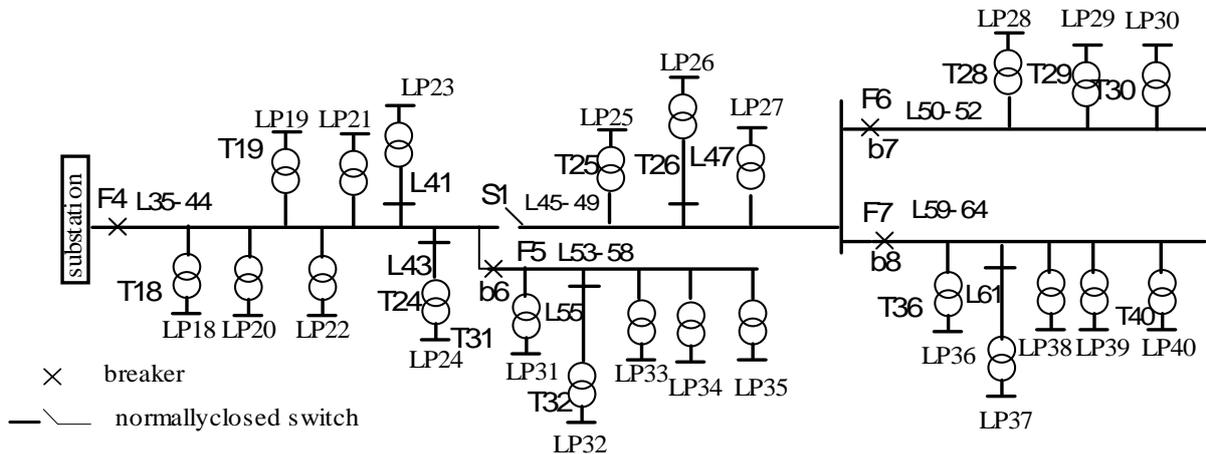
Figure 1. Complete Single line diagram of RBTS.
