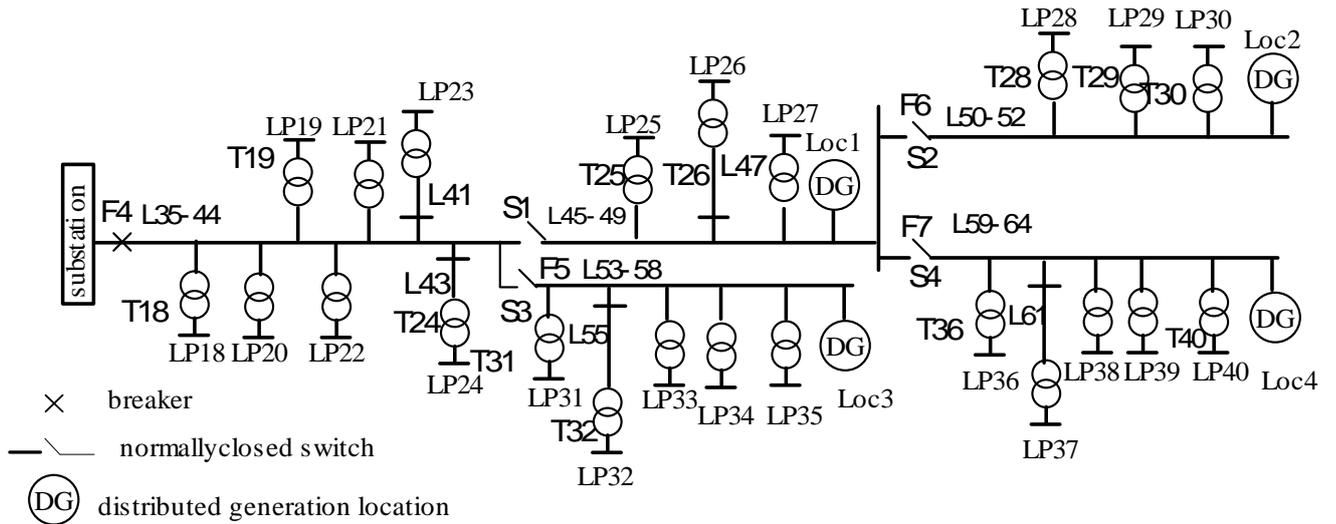
Figure 3. Complete Single Line Diagram of RBTS.
