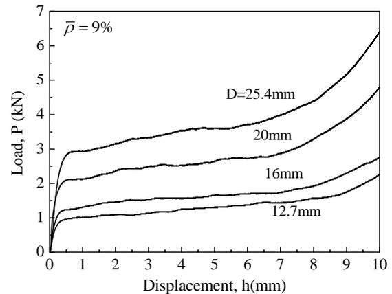
Figure 3.  $P-h$  curves of Al foam under different diameters of the flat-end cylindrical indenters.
