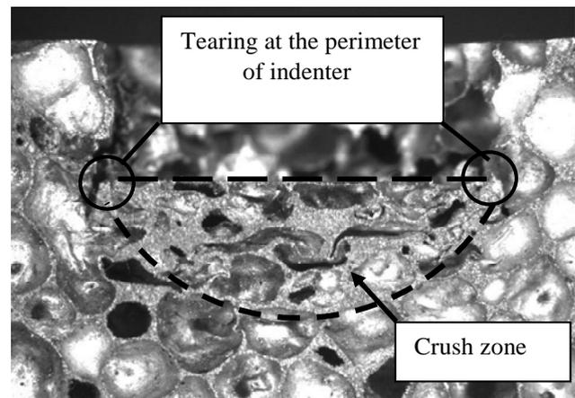
Figure 7. Cross-sectional morphology of Al foam after indentation.
