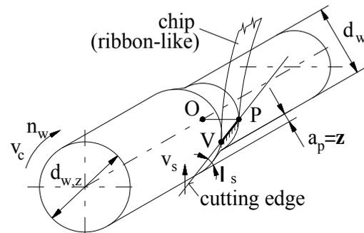
Figure 2. The principle of material removal in rotational feed turning.
