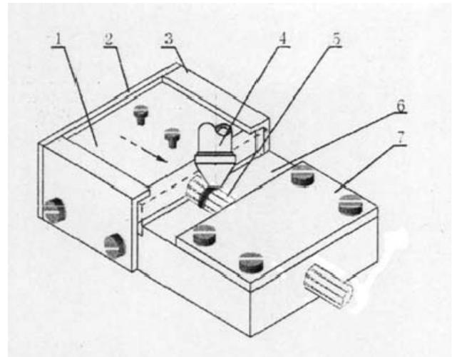
Figure 2. Aluminum alloy / aluminum matrix composites welding fixtures (1 dynamic pressure board ; 2 backboard; 3 right and left board; 4 plasma torch; 5 composite; 6 the base; 7 static pressure board).
