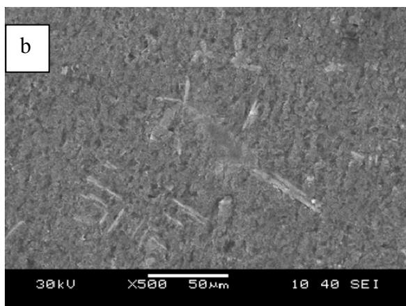
Figure 8. Microstructure of weld during  $I=180A$  (a) Weld center; (b) Weld edge.
