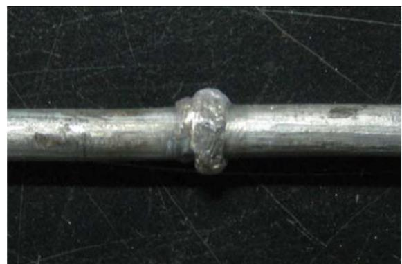
Figure 3. Appearance of joint during  $I=150\text{A}$ .
