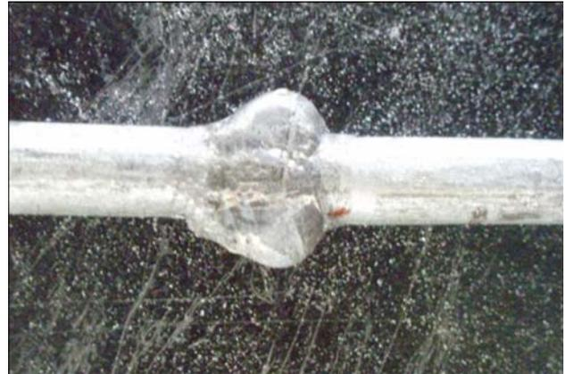
Figure 6. Joint form during  $I=180A$ .
