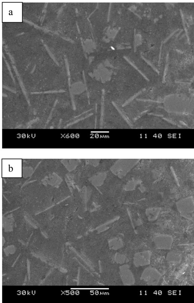
Figure 5. The microstructure of weld during  $I=150A$  (a) Weld center; (b) Weld edge.
