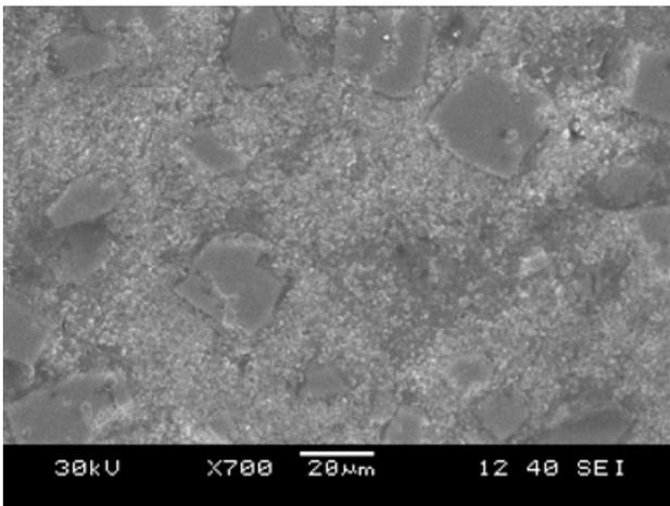
Figure 1. The microscopic photos of the Al-ZrO<sub>2</sub> System composite synthesized by XD method.
