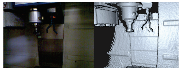
Figure 7 Raw scan data from ReconstructMe
