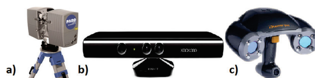
Figure 2 a) Farp LS 880, b) Kinect, c) ZScanner 700
