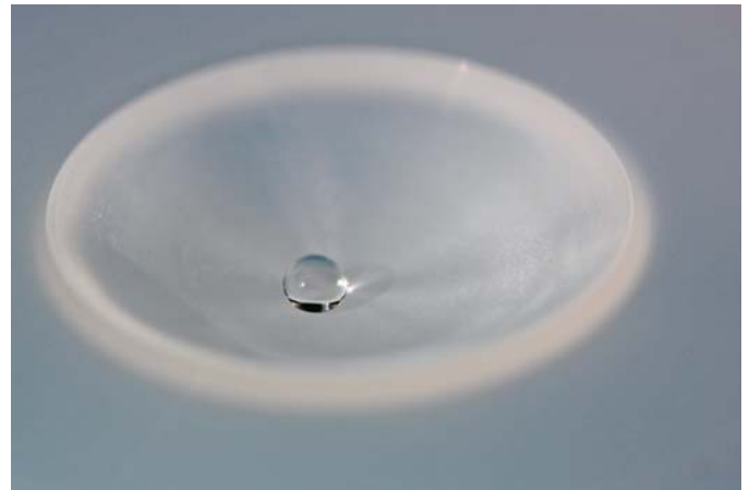
FIGURE 2 – Part with water repelling surface – produced in a one-step injection moulding process ( IKV )
