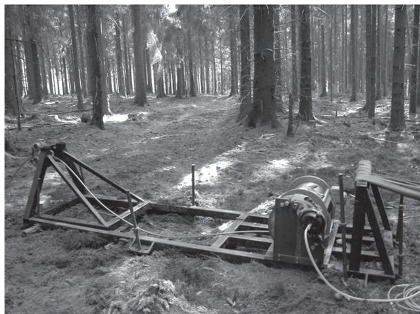
**Fig. 2** Winch to apply the loads for traction measurements installed on a skidding lane
