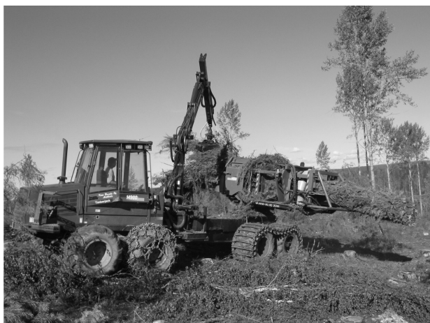
Fig. 1 Forwarder-mounted Timberjack/John Deere 1490D logging residue bundler operating in a clear-cut area
