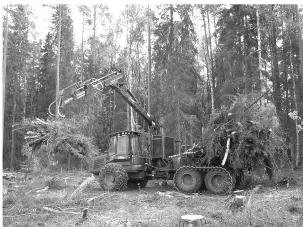
Fig. 4 Forwarding of pre-piled logging residues with a heavy forwarder at the stand
