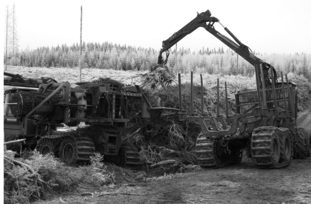
Fig. 3 Separate loading of logging residues with the Valmet 840.3 forwarder to the feeding table of the John Deere 1490D logging residue bundler (working methods I and II)
