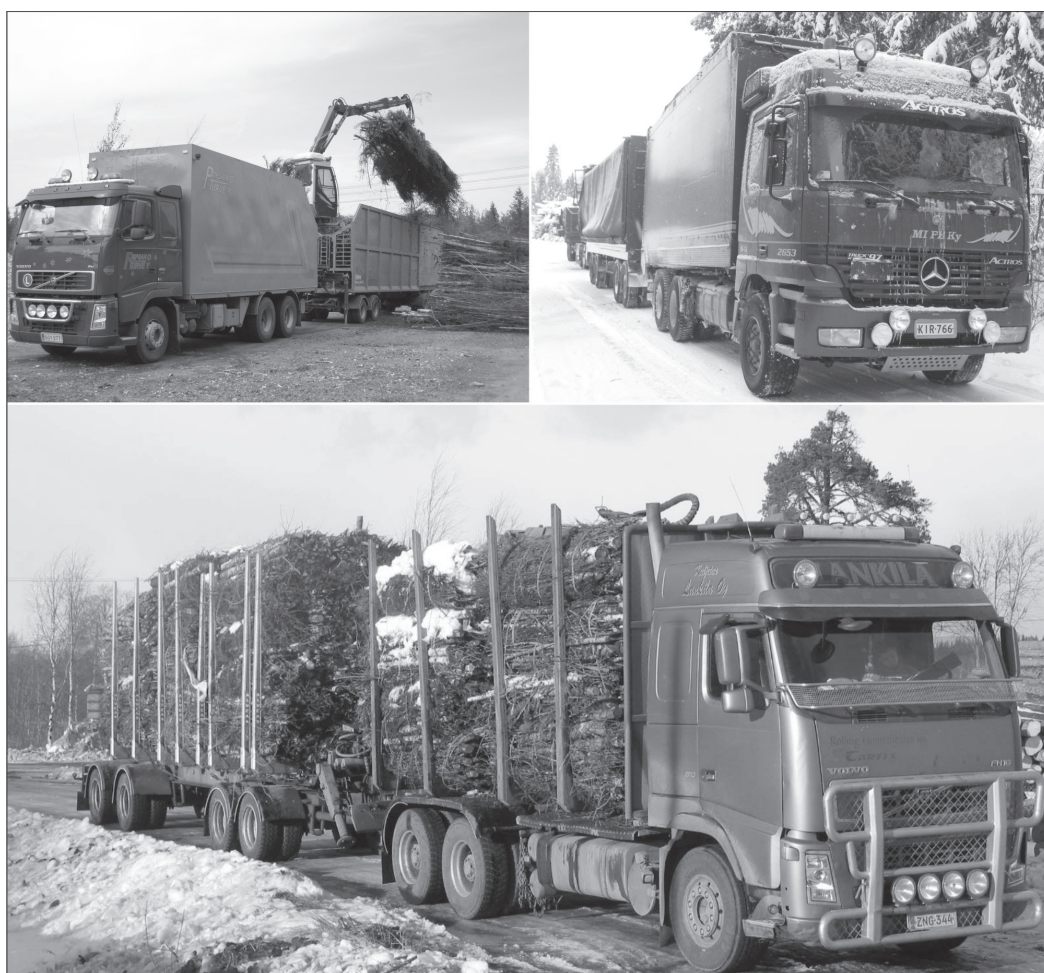
Fig. 2 A biomass truck equipped with solid side panels and bottom (left up), a standard chip truck (right up), and a standard timber truck (down) Slika 2. Kamion za prijevoz biomase s obloženim tovarnim prostorom (gore lijevo), uobičajeni kamion za prijevoz iverja (gore desno) te kamion za prijevoz drva (dolje)
