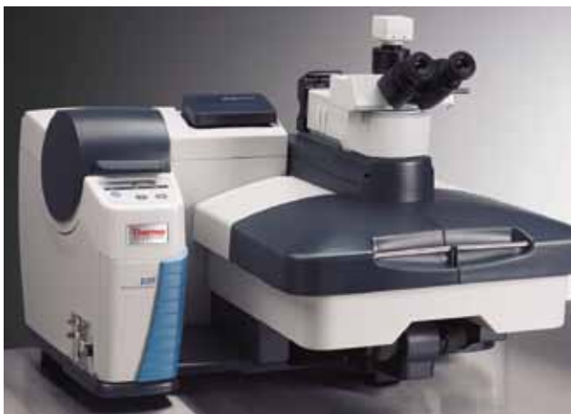
45 Jedan od modela Ramanova mikroskopa One of the Raman microscope models
