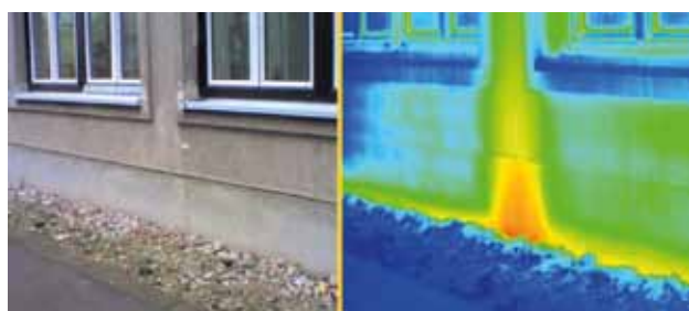
28 Zid zgrade i isti zid gledan termovizijskom kamerom pokazuje mnogo slabije termičko zračenje u zoni koja je zbog sakrivene vlage hladnija. (Preuzeto iz: B. Srša, nav. dj.) Building wall and the same wall seen through a thermo-visual camera shows considerably lower thermal radiation in the zone which is colder due to hidden humidity. (taken from: B. Srša, op. cit.)
