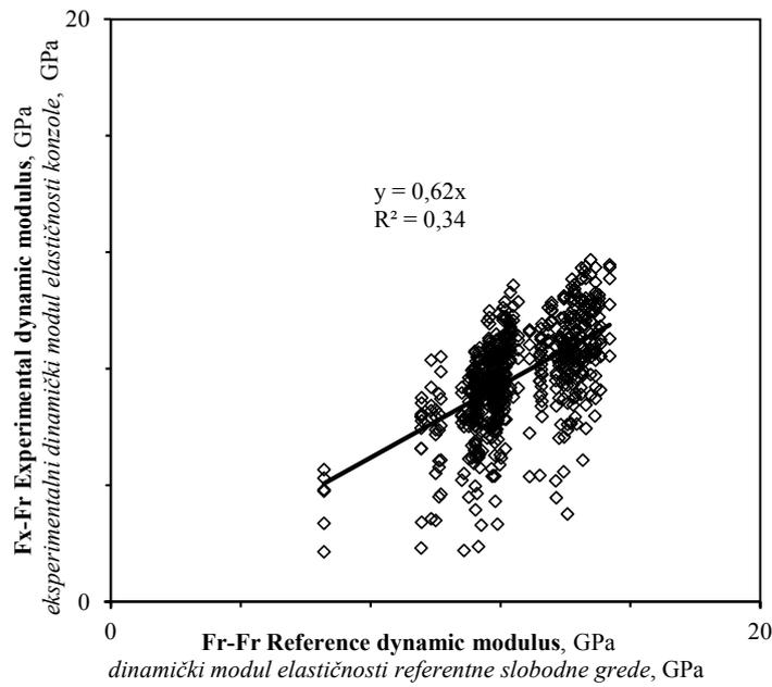
**Figure 6** Experimental unmodified fixed-free versus reference free-free dynamic modulus
