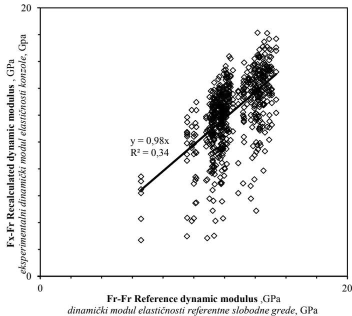
**Figure 7** Recalculated fixed-free versus reference free-free dynamic modulus
