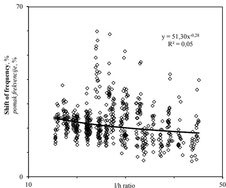
**Figure 4** Frequency shifts versus  $l/h$  ratio of specimens in the stepwise scenario
