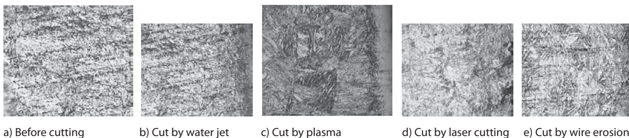
Figure 5 Micro structure photos of cutting border and surfaces of the sample cut by different cutting methods
