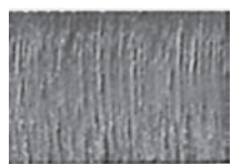
Figure 2 Photo of surface of shear of the sample cut by laser
