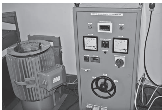
Figure 4 View of electro-magneto-hydro pump used for collecting platinum in lead
