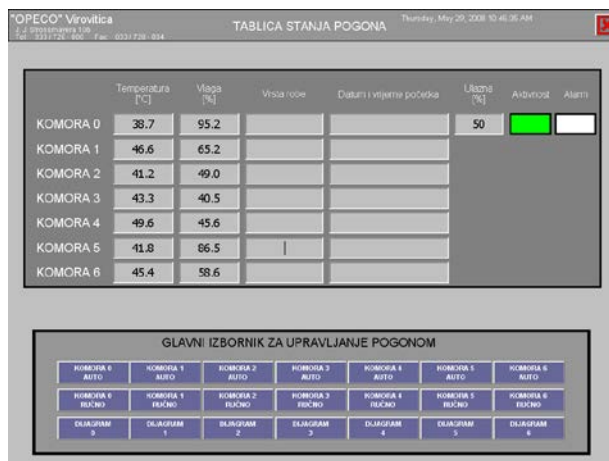
Figure 7. Sample of SCADA screens for Brick drying automation system
