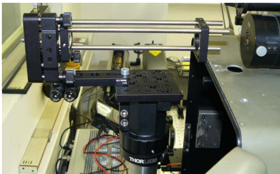
Fig. 6 Telescope assembly at interferometer aperture. The beam exiting the optical fibre is first collimated and then focused onto input aperture of interferometer.
