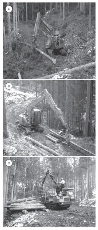
**Fig. 2** Operational system with grapple-loader bunching (A), processor processing (B), and forwarder forwarding (C)
