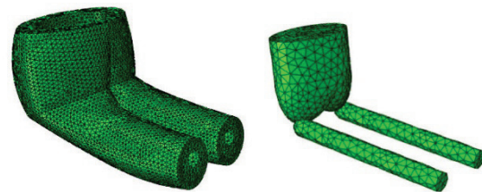
Figure 11 The FEA mesh model of the seating human
