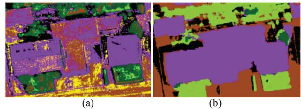
**Figure 2** Refinement of the classification result: (a) Classification result, (b) Refined result: purple - building class, yellow - road, brown - bare ground, light green - grass, dark green - tree, black - shadow
