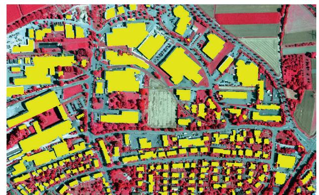
**Figure 17** Detected buildings (yellow) from combination of results
