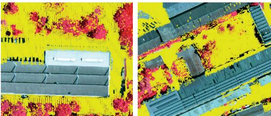
Figure 3 LIDAR DTM overlaid on an orthoimage
