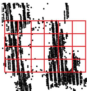
Figure 4 Density calculation over LIDAR DTM. Overlaid grids (red) and LIDAR DTM points (black).
