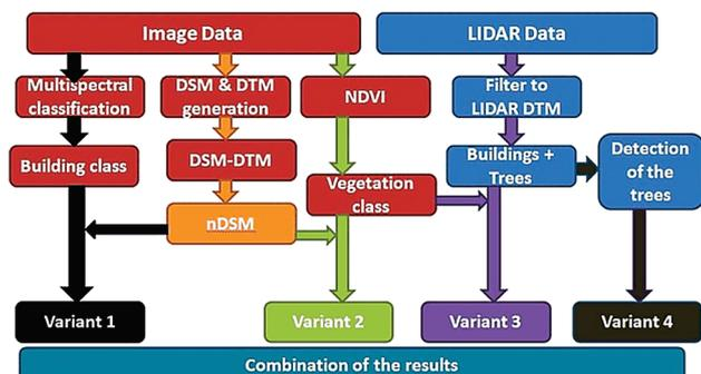
Figure 1 Workflow of the building detection, red indicates the items related to the image data, blue LIDAR data, orange is nDSM, and the results of different approaches have different colours
