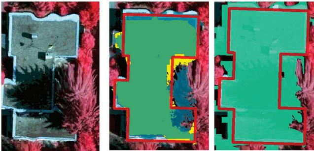
**Figure 15** Combination of the results, Left: example on the orthoimage, middle: intersection of the variants 1 and 2, Red outline: reference data, blue: result from variant 1 yellow: result from variant 2 green: intersection of the result from variants 1 and 2, right: green: union of the results from variant 3 and 4, red outline: Reference data.
