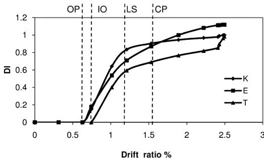
Figure 5 Variations of structural damage indexes at different performance levels of the six-story frame
