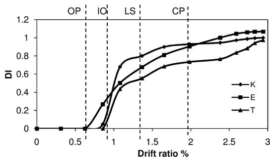
Figure 4 Variations of structural damage indexes at different performance levels in the three-story frame
