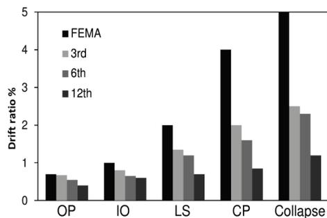
**Figure 9** Comparison of drift in different performance levels with FEMA
