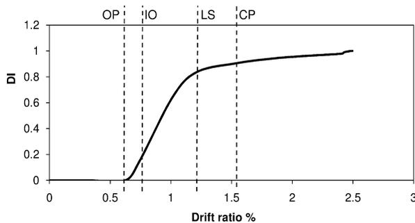
Figure 3 Variations of structural damage index at different performance levels for six-story frame building
