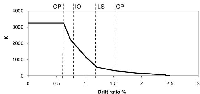
Figure 2 Variations of structural stiffness at different performance levels for six-story frame building
