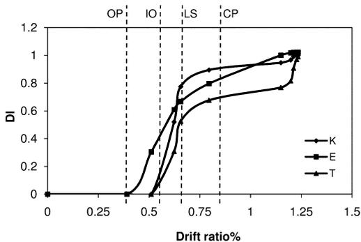
Figure 6 Variations of structural damage indexes at different performance levels of the twelve-story frame
