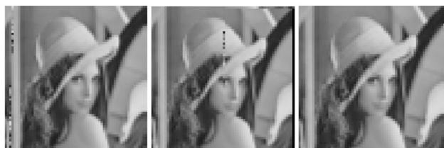
a) Error at the beginning of sequence b) Error in the middle of sequence c) Error at the end of sequence
