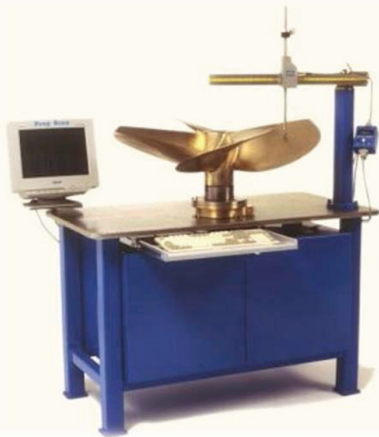
Slika 5. Prop Scan sustav za ispitivanje vijka [6] Figure 5. Prop Scan system for testing propellers [6]
