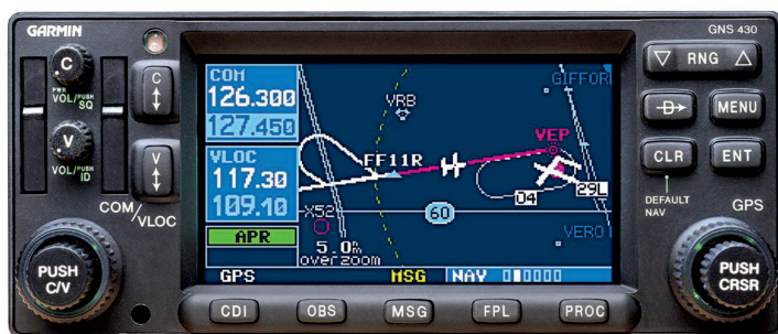
Figure 5. Garmin GNS 430 GPS receiver
