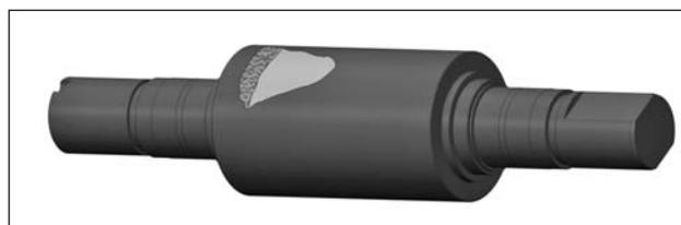
**Figure 1** A Cat's Tongue Spall visible on working roll surface layer
