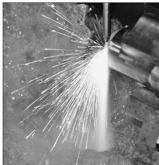
Figure 4 AWJ Turning process of Titanium Workpiece
