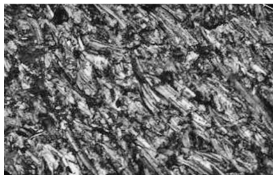
Figure 12 Machined Titanium surface using AWJ, (Zoom 20 x)
