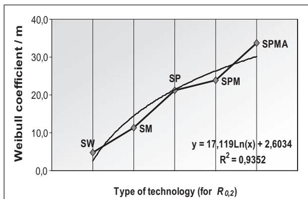
Figure 3 Weibull coefficient of AISi17Cu5 cast alloy for yield strength  $R_{0,2}$  as a function of applied technologies
