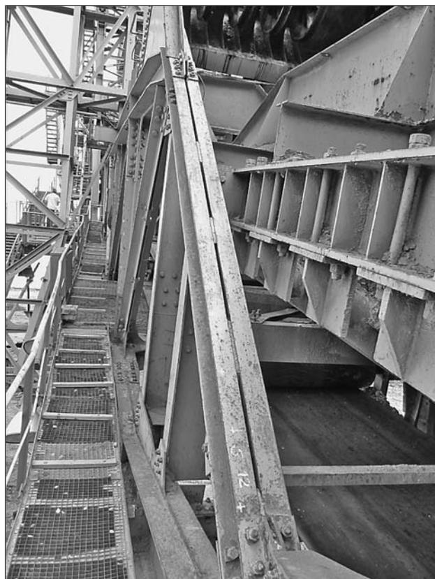
Figure 2 The deformed element of the excavator arm
