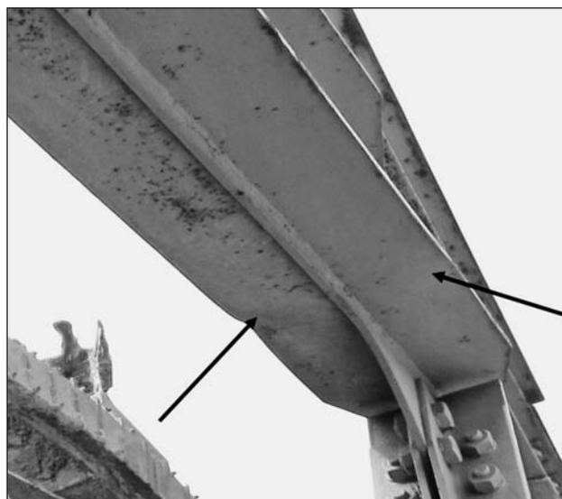
Figure 3 The mode of deformation of the excavator arm element
