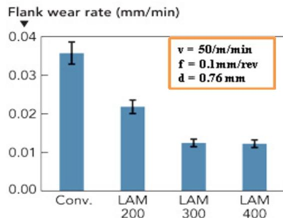
Figure 4. Tool wear vs. temperature [58].
