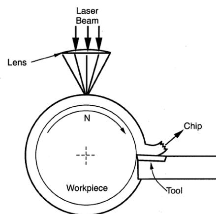
Figure 1. A schematic representation of laser assisted machining [59].
