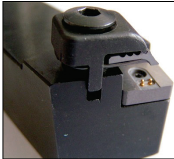
Figure 2 Tool holder with contacts for the transmission of electrical signals
