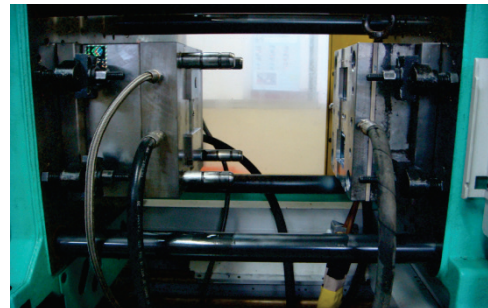
Figure 12 The insert type induction heating tool set up in an Arbuge 320C machine
