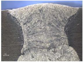
Fig. 7 Macrostructure of the welded joint
