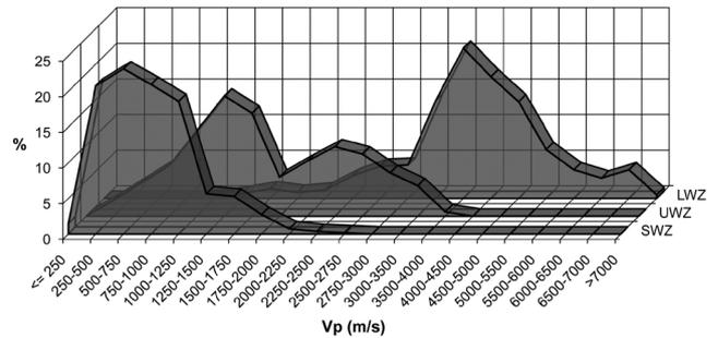
Figure 11: The distribution of the primary seismic waves velocities ( $V_p$ ) in different weathering zones in limestones across the AdCP.
