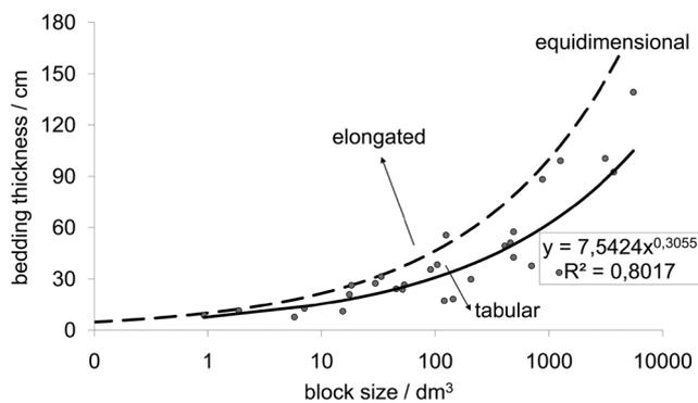
**Figure 5:** Correlation of the average bedding discontinuity spacing and block size in the Croatian carbonate rocks from the Middle Triassic to the Oligocene (continuous line). Dashed line represents ideal, calculated equidimensional blocks.
