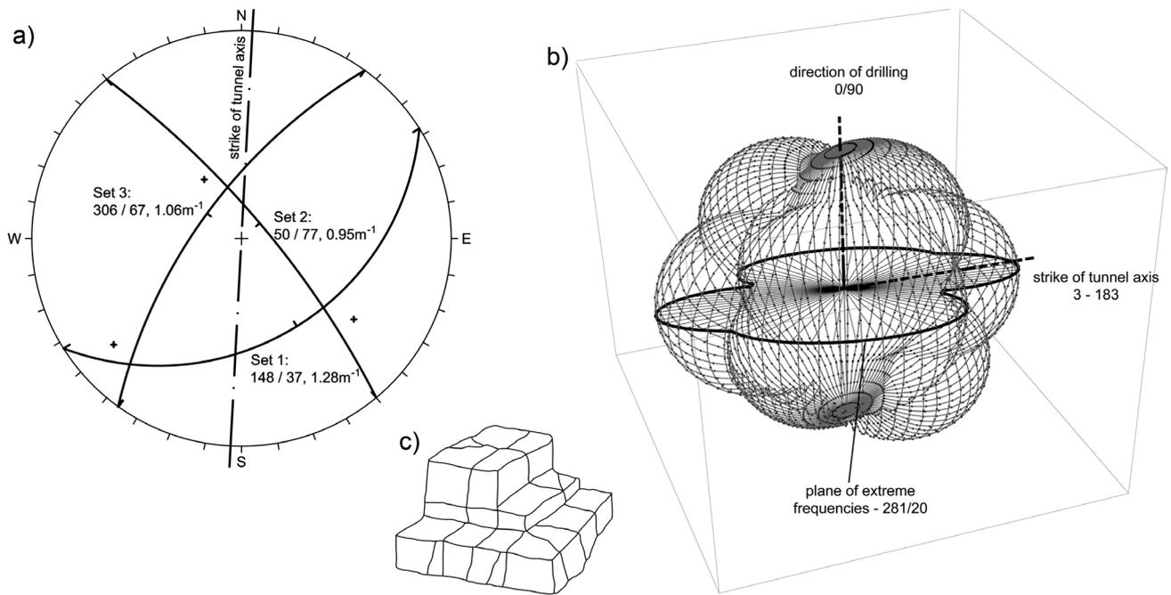
**Figure 6:** The "Mala Kapela" Tunnel – structural unit A (3 sets): a) Equal angle lower hemispherical projection of example data, b) three-dimensional locus of discontinuity frequency with plane of extreme (range) frequencies, c) equidimensional blocks.
