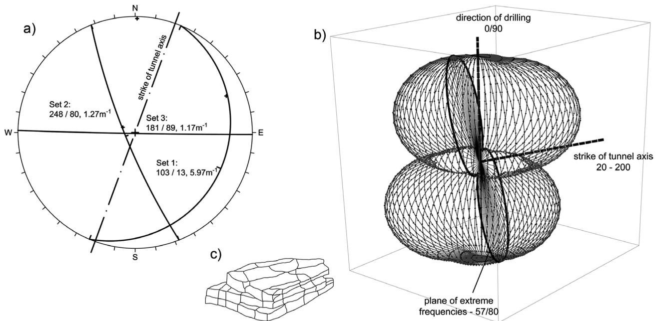
**Figure 7:** The "Brinje" Tunnel – structural unit E (3 sets): a) Equal angle lower hemispherical projection of example data, b) three-dimensional locus of discontinuity frequency with the plane of extreme frequencies, c) tabular blocks.
