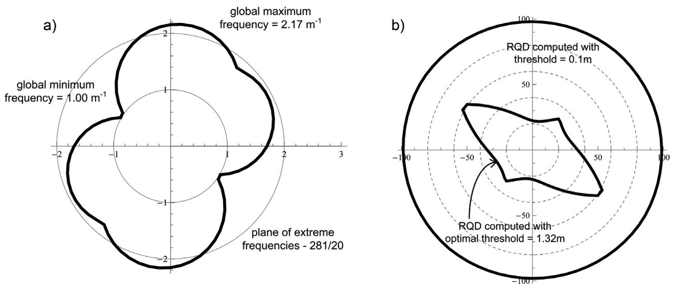
**Figure 8:** The "Mala Kapela" Tunnel – structural unit A (3 sets): a) Polar plot of discontinuity frequency; b) polar plot of RQD using customary threshold value 0.1 m and optimal threshold value.
