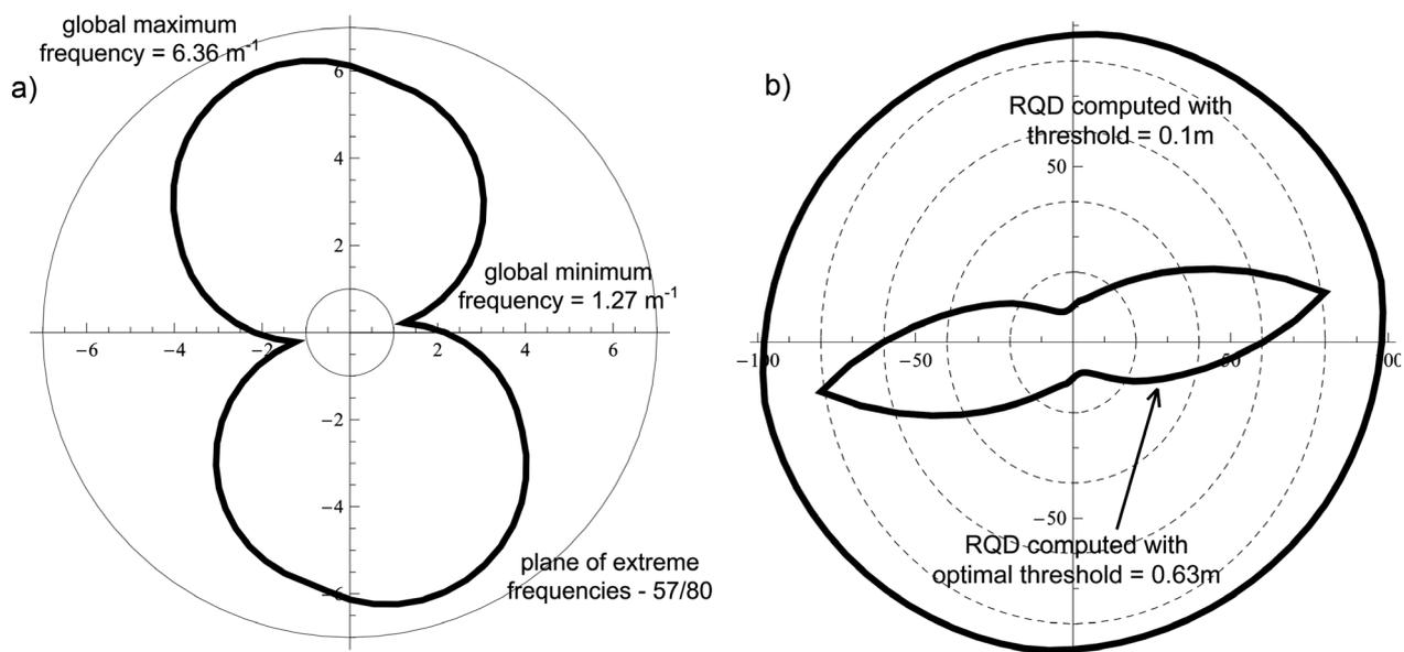
**Figure 9:** The "Brinje" Tunnel – structural unit E (3 sets): a) Polar plot of discontinuity frequency, b) polar plot of RQD using customary threshold value 0.1 m and optimal threshold value.
