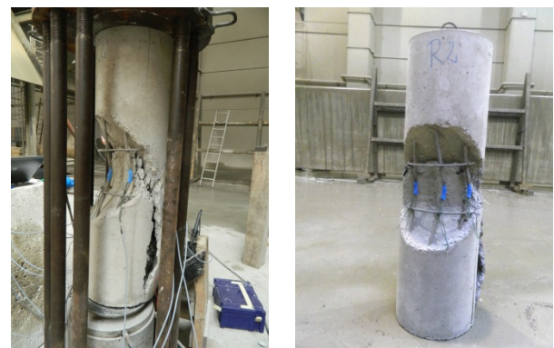
Figure 3 Implementation of experiment on model of circular cross section, with oblique damage, model with damaged depth R (radius)
