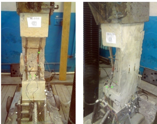
Figure 2 Implementation of experiment on models of rectangular cross section, with oblique damage.
